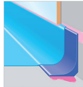
Prefabricated concave moulding made of epoxy resin for tiled wall and coated floor surface
